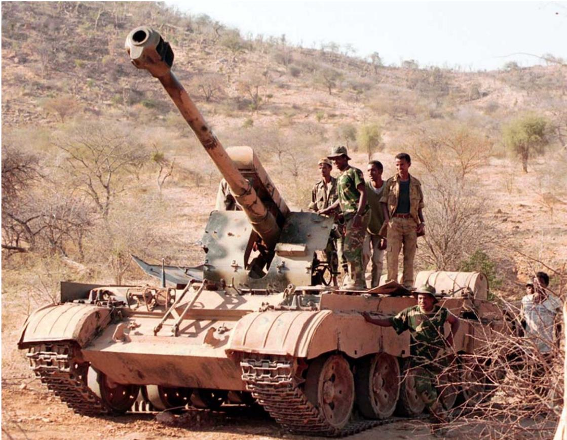
*A self propelled gun made by assembling a 122mm MI 1963D30 gun- howitzer on the hull of a T54/55*
